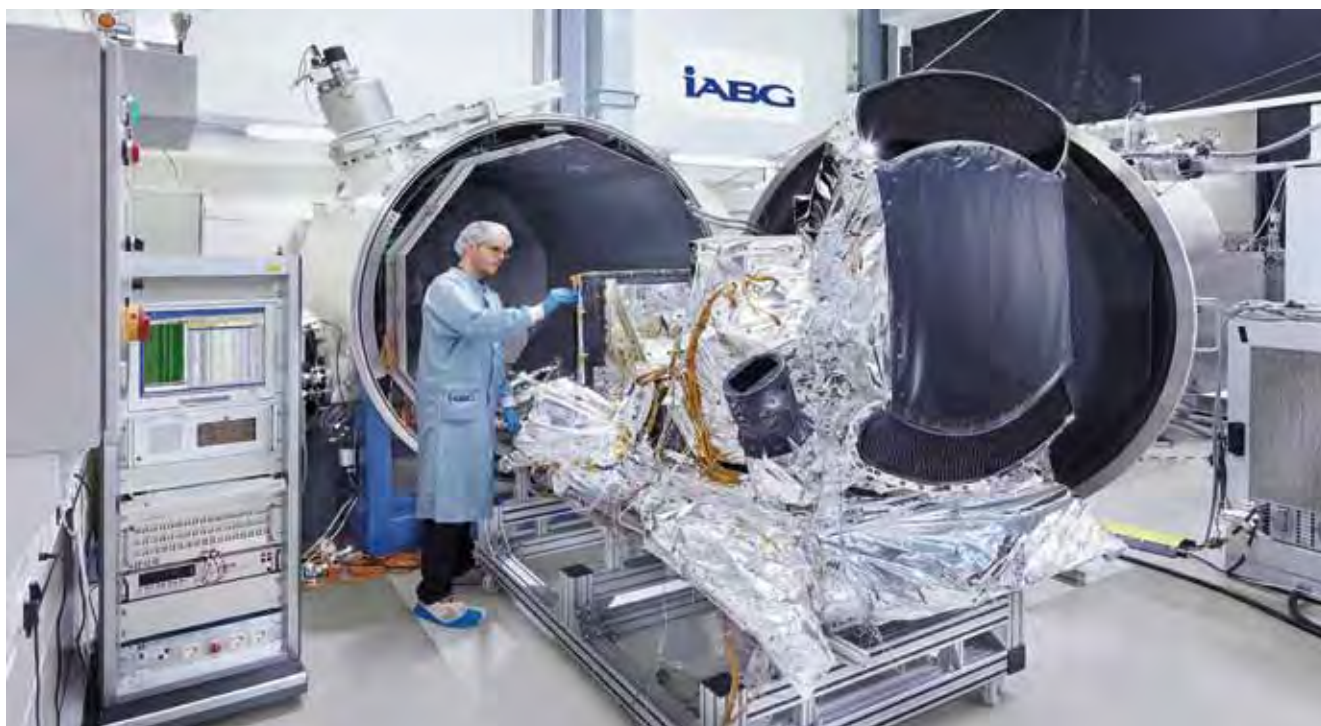
Figure 6.3. The SLSTR Optical Scanning Unit. (IASG)
