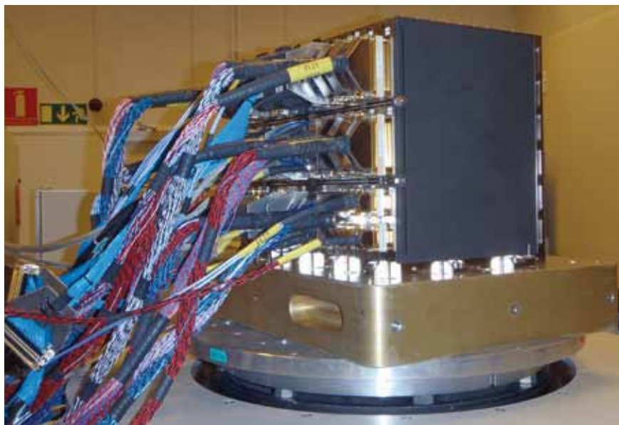
Figure 5.7. The Satellite Management Unit on the shaker, prepared for vibration qualification. (RUAG, Sweden)
