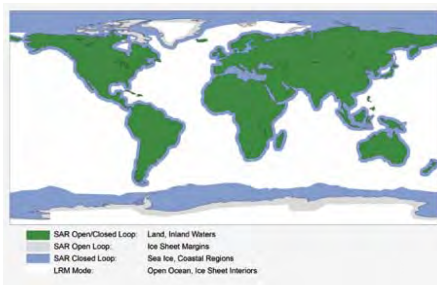
Figure 4.4. Baseline SAR/LRM mode map for the SRAL instrument.
