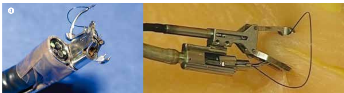
❸ 趙偉仁教授示範以內鏡手術機械人進行內鏡黏膜下剝離術 Prof. Philip Chiu demonstrates the use of the endoscopic surgical robot to perform ESD
