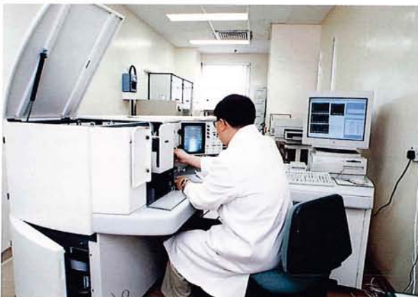
FACS Vantage flow cytometer being used to determine NPC tumour characteristics such as the percentage of dividing cells present in a biopsy specimen
