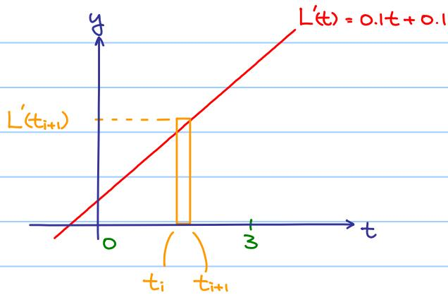
Area of the rectangle =  $L'(t_{i+1}) \times (t_{i+1} - t_i) \approx \text{change of CO between } t_i \text{ and } t_{i+1}$
