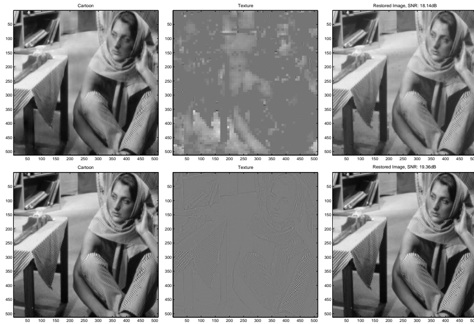
Figure 3. Zooming. The reconstruction image for Model 1 (top row) and Model 2 (bottom row).
