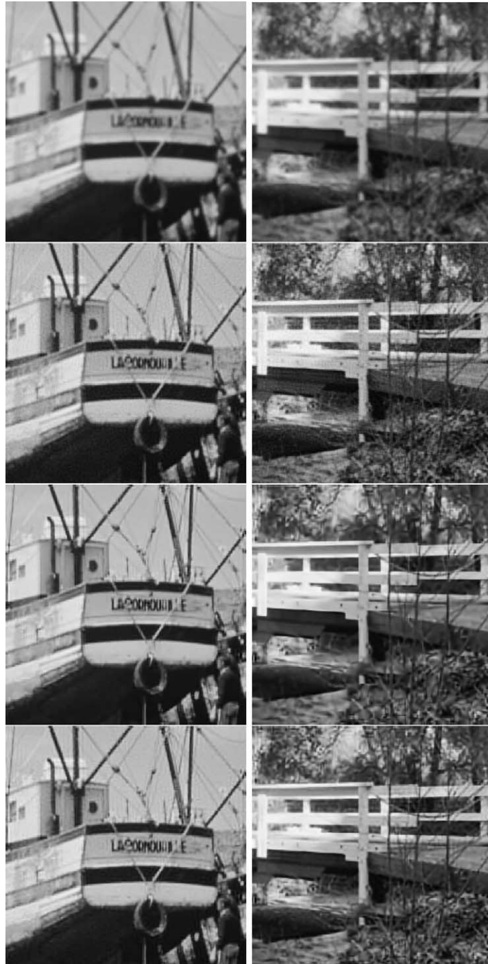
Fig. 4. 4 \times 4 sensor array without displacement error at SNR of 30 dB. The images (from top to bottom) are: observed high-resolution image, results with LS, WA, and TF, respectively.
