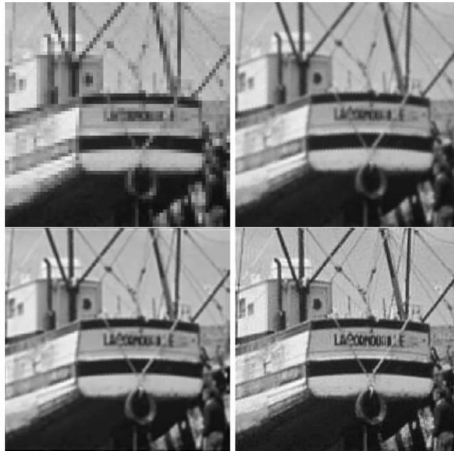
Fig. 5. 4 \times 4 sensor array with displacement error at SNR of 30 dB for “boat” image. A low-resolution image from the (0,0) sensor (top-left); observed high-resolution images (top-right); reconstructed images with WA (bottom-left); and TF (bottom-right).
