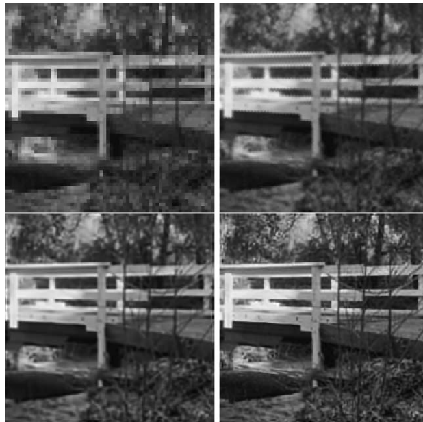
Fig. 6. 4 \times 4 sensor array with displacement error at SNR of 30 dB for “bridge” image. A low-resolution image from the (0,0) sensor (top-left); observed high-resolution images (top-right); reconstructed images with WA (bottom-left); and TF (bottom-right).
