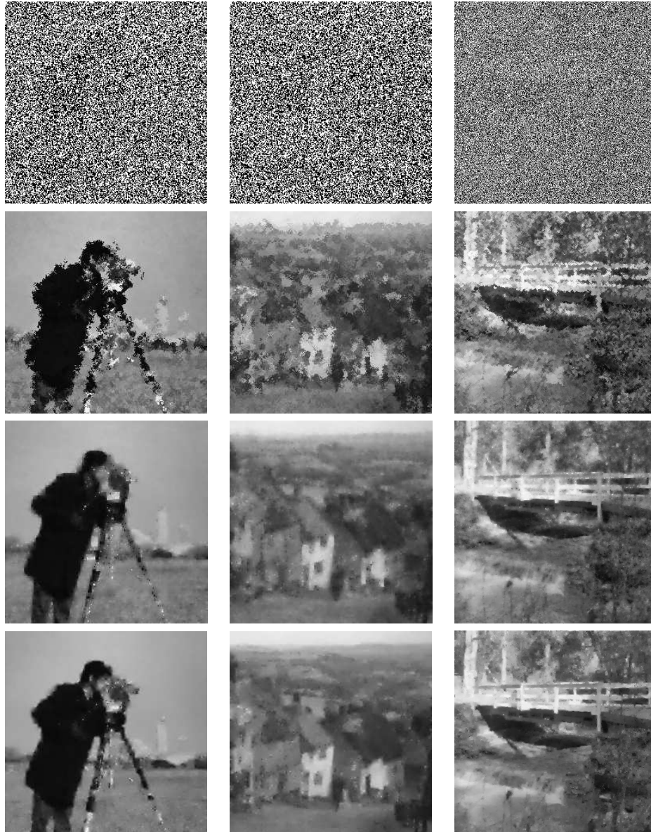
Figure 3: From top to bottom: images corrupted with 90% salt-pepper noise, restored by AMF, restored by 2-phase variational method [7], and restored by Algorithm 2.
