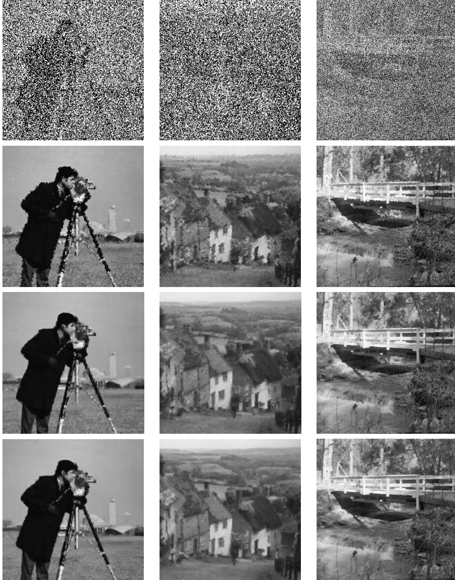
Figure 2: From top to bottom: images corrupted with 70% salt-pepper noise, restored by AMF, restored by 2-phase variational method [7], and restored by Algorithm 2.
