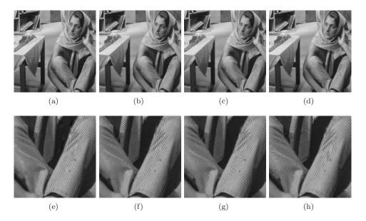
FIGURE 2. The results of tight frame based inpainting algorithms. The upper row shows the restored images by (from left to right) (12) with  $\kappa = 0$ ,  $\kappa = 1$ ,  $\kappa = \infty$  and by the algorithm in [6] (i.e.(5)). The PSNR values are 33.98dB, 34.47dB, 34.75dB and 31.89dB respectively. The bottom row shows the corresponding zoomed images.
