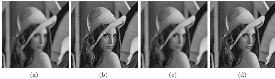
FIGURE 3. Lena image blurred with out-of-focus kernel of radius 3, and then corrupted by impulse noise with s = 30\% for Figs (a) and (b), and r = 25\% for Figs (c) and (d). Fig (a) is the result of AMF and Fig (b) is the result by first applying AMF and then minimizing (3)–(4) with \varphi(t) = \sqrt{t^2 + 10^{-4}} and \beta = 0.01 . Fig (c) is the result of ACWMF and Fig. (d) is the result by first applying ACWMF and then minimizing (3)–(4) with \varphi(t) = \sqrt{t^2 + 10^{-4}} and \beta = 0.01 .
