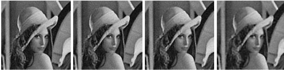
FIGURE 11. Lena image blurred with out-of-focus kernel of radius 3, and then corrupted by Gaussian noise with \sigma = 5 and random-valued impulse noise with r = 10\% , 25\% , 40\% , and 55\% respectively. From left to right: The restored image by our method with PSNRs 27.2dB, 27.0dB, 26.7dB, and 25.6dB respectively. The parameters we used are [\alpha = 0.05, \beta = 0.05, \epsilon = 0.0002] , [\alpha = 0.01, \beta = 0.005, \epsilon = 0.0002] , [\alpha = 0.01, \beta = 0.005, \epsilon = 0.0002] , [\alpha = 0.01, \beta = 0.01, \epsilon = 0.0001] respectively. The functional minimized is (13) for p = 2 for s = 10\% and (13) for p = 1 for others according to Table 2. The \tilde{\sigma} is 6.5, 7.0, 8.4 and 11.9 respectively.
