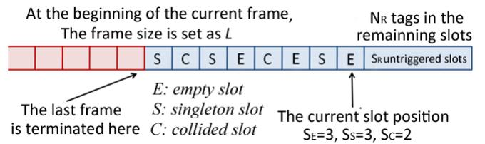
Fig. 3. The reading process of Gen-2 algorithms.
