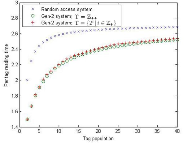
Fig. 4. The average contention time per tag using the optimal reading strategy.
