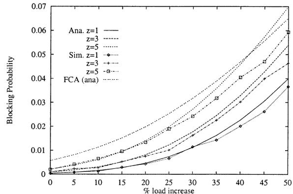
**Fig. 4** Performance of CGD analysis in a 20-cell linear network with base traffic load 150 calls/hr/cell and mean call holding time 3 minutes. The total number of voice channels per cell is 15. The number of voice channels per carrier varies with  $z = 1, 3$  and 5 respectively.
