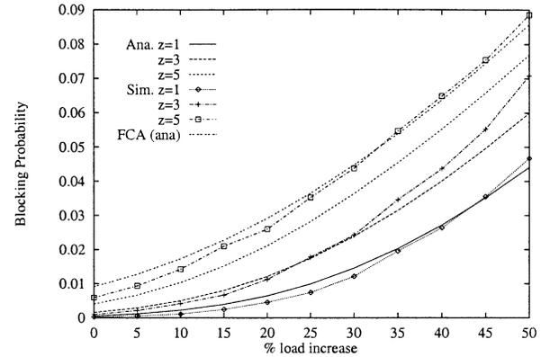
**Fig. 10** Performance of phantom cell analysis in a 49-cell planar network with 160 calls/hr/cell and mean call holding time 3 minutes. The total number of voice channels per cell is 15. The number of voice channels per carrier varies with  $z = 1, 2$  and 3 respectively.
