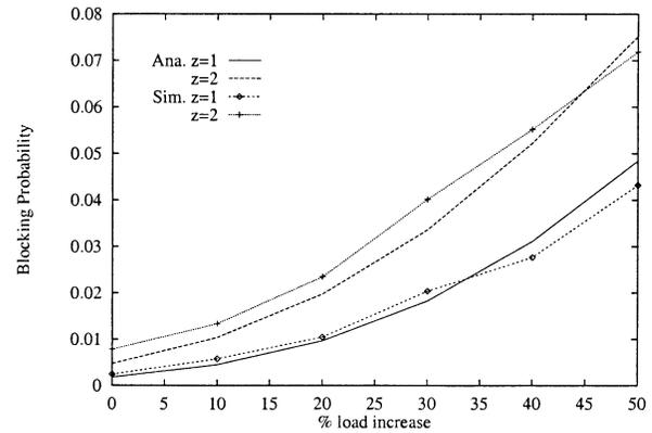
**Fig. 7** Performance of CGD analysis in a 49-cell planar network with base traffic load 50 calls/hr/cell and mean call holding time 3 minutes. The total number of voice channels per cell is 6. The number of voice channels per carrier varies with  $z = 1$  and 2 respectively.
