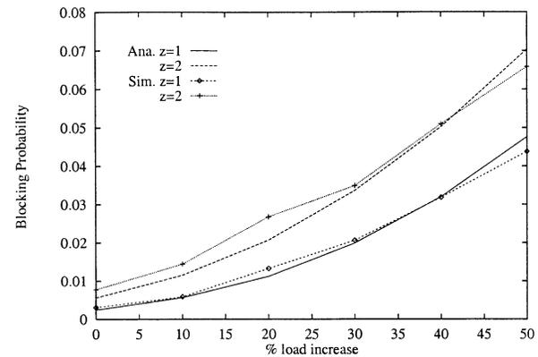
**Fig. 8** Performance of CGD analysis in a 49-cell planar network under non-uniform traffic distributions (shown in Fig. 6) with mean call holding time 3 minutes. The total number of voice channels per cell is 6. The number of voice channels per carrier varies with  $z = 1$  and 2 respectively.
