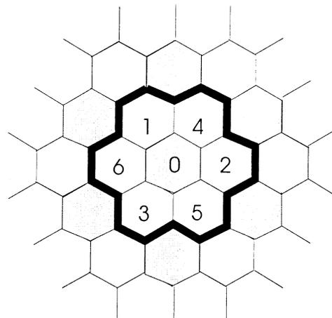
**Fig. 3** A planar cellular system with three-cell reuse pattern. Cells 0 to 6 form a decoupled system for cell group decoupling analysis and phantom cell analysis.
