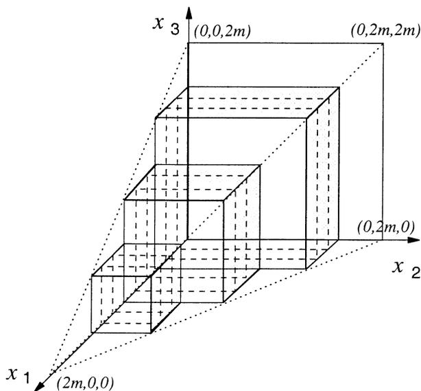
**Fig. 2** A three-dimensional markov chain for describing the state space of a decoupled linear system with  $z = 3$  voice channels per carrier.
