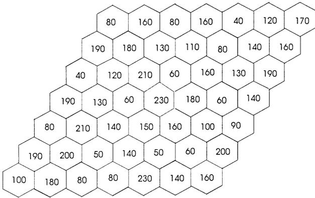
**Fig. 9** A 49-cell cellular system with three-cell channel reuse pattern for phantom cell analysis. The number inside each cell represents the basic traffic load (in calls/hr) under the non-uniform traffic distribution.
