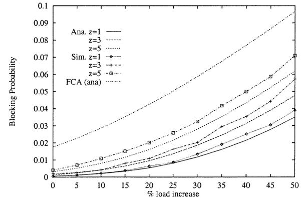
**Fig. 11** Performance of phantom cell analysis in a 49-cell planar network under non-uniform traffic distributions (shown in Fig. 9) with mean call holding time 3 minutes. The total number of voice channels per cell is 15. The number of voice channels per carrier varies with  $z = 1, 2$  and 3 respectively.
