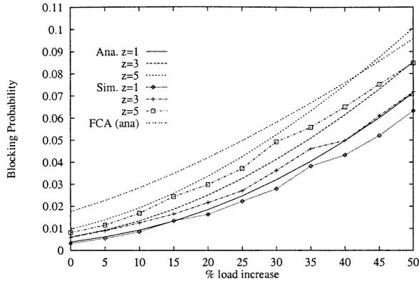
**Fig. 5** Performance of CGD analysis in a 20-cell linear network under non-uniform traffic distributions with mean call holding time 3 minutes. The total number of voice channels per cell is 15. The number of voice channels per carrier varies with  $z = 1, 3$  and 5 respectively.
