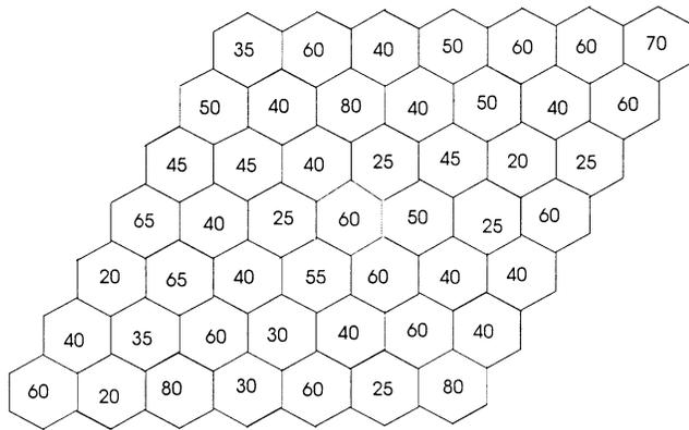
**Fig. 6** A 49-cell cellular network with three-cell channel reuse pattern for CGD analysis. The number inside each cell represents the basic traffic load (in calls/hr) under the non-uniform traffic distribution.
