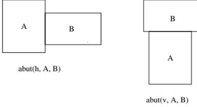
Figure 3: Abutment Constraints.
