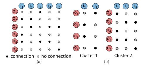
**Fig. 4.** (a) Connection matrix W of a sparse neural network with five input neurons  $\{i_1, ..., i_5\}$  and six output neurons  $\{o_1, ..., o_6\}$ ; (b) pruned connection matrices of the two clusters  $W_1$  and  $W_2$  generated by hierarchical clustering.
