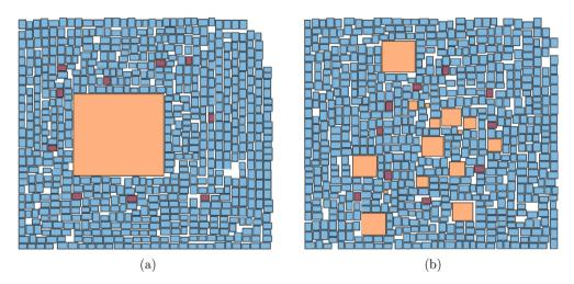
Fig. 8. Floorplan examples of the neural network  $b_1$  generated by (a) "SC + NLP + MH" (area: 1.09 mm<sup>2</sup>); (b) "FC + NLP + MP" (area: 1.02 mm<sup>2</sup>).
