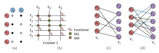
**Fig. 6.** (a)  $W_1$  of cluster 1; (b) an example of the mapped memristor crossbar  $C_1$  for  $W_1$ ; (c) a bipartite graph of  $W_1$  to  $C_1$  under  $A_c = [1, 2]$ , in which a matching cannot be solved; (d) a bipartite graph of  $W_1$  to  $C_1$  under  $A_c = [3, 2]$  and the maximum bipartite matching result  $A_r = [2, 1, 3, 5]$  (blue lines). (For interpretation of the references to colour in this figure legend, the reader is referred to the Web version of this article.)
