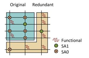
Fig. 5. An example of the mapped memristive crossbar for  $W_1$ .
