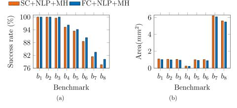
Fig. 7. Comparison between "SC + NLP + MH" and "FC + NLP + MH" on (a) success rate and (b) area.
