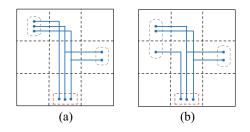
Fig. 4. Illustration of source-to-sink distance for signal bits. (a) Example of equivalent distance for all bits. (b) Example of interbit distance deviation.
