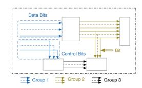
Fig. 1. Example of on-chip signal groups.
