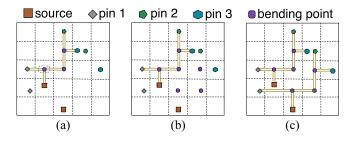
Fig. 6. Equivalent topology generation example: (a) Pin mapping through similarity vector. (b) Bending points aligning. (c) Topology generation by connecting mapping pins and points.
