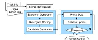
Fig. 2. Overall streak flow.
