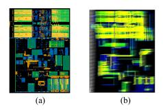
Fig. 12. Routing congestion map for Industry6. (a) Manual design result. (b) Streak result.
