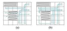
Fig. 7. Example of blocked routing instance. (a) Routing of some bits blocked by obstacles. (b) Multiple topology selection for each cluster.
