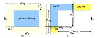
**Fig. 4** (a)No matter how to move the module, dark area can not insert level-shifter, while blank area is Potential White Space(PWS) of  $R_j$  (b)1st and 2nd Feasible Region of  $FR_{ij}$ .
