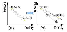
**Fig. 3** For a module, when number of legal working voltages is 2, (a)original DP-curve, (b)modified DP-curve, adding the power and delay of level-shifter.
