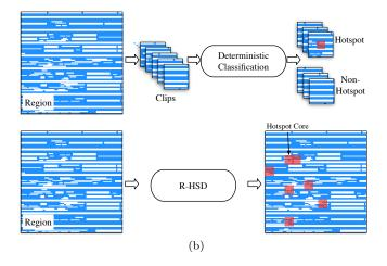
Fig. 2.: (a) Conventional hotspot detection flow vs. (b) Region based hotspot detection flow as presented in [20].
