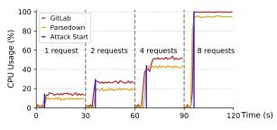
Fig. 5: Server-side CPU usage over time under attacks on GitLab and Parsedown.
