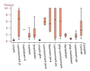
**Fig. 4:** Compilation time of Markdown compilers under attack inputs of the size of 50,000 characters and a 10-second maximum threshold. The middle lines in the boxes represent the corresponding median values.
