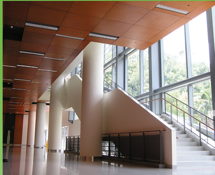
High glass allowing natural light into the lobby, complete with photo sensors for light fittings
