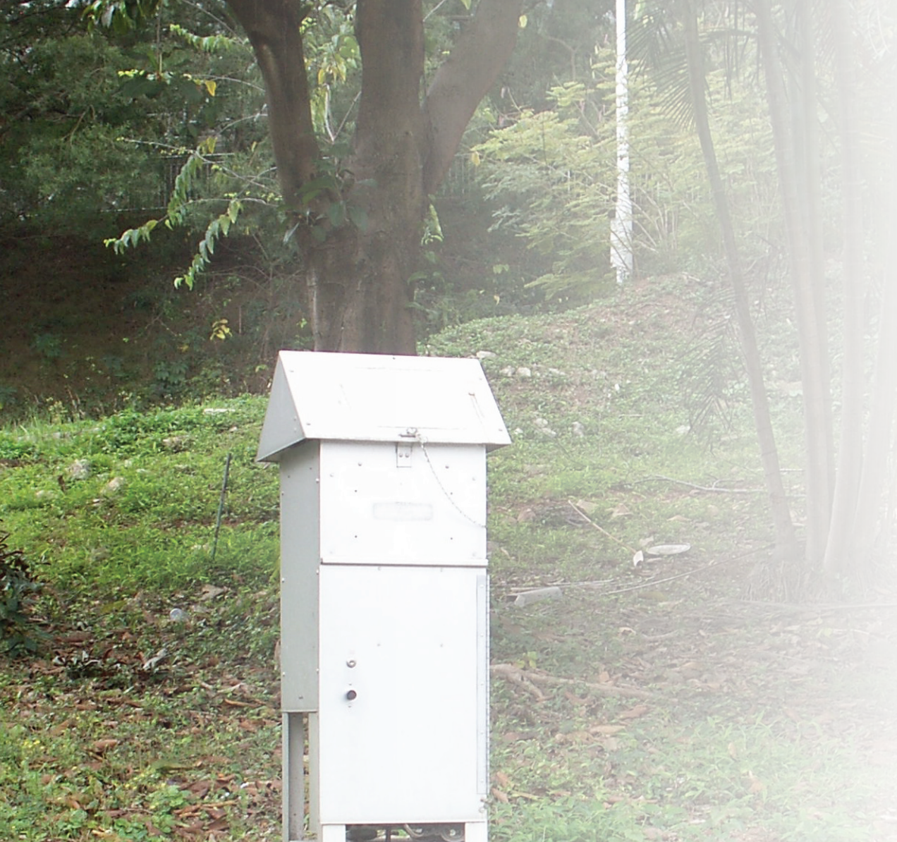
A TSP sampler is installed near Residence 10 to monitor the dust level
