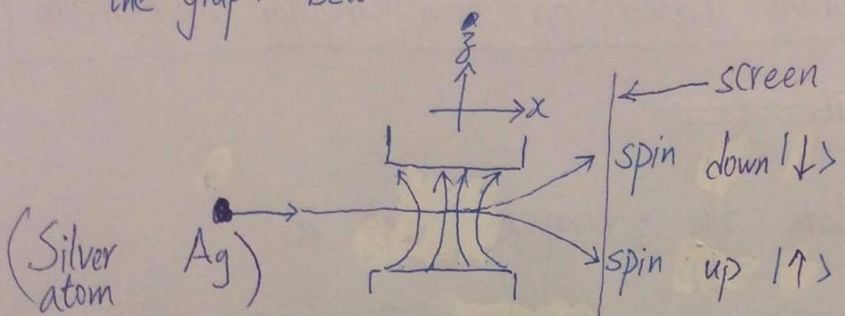
A silver atom is shot towards the <sup>inhomogeneous</sup> magnetic field, nearly perpendicular to the motion. Depending on the direction of the spin, the silver atom is bent either upwards or downwards by the "magnetic force" acting on the spin. of outermost electron
