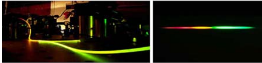
Fig. 1. Fiber-optical horizons. (A) A light pulse in a fiber slows down infrared probe light, attempting to overtake it. The diagrams below are in the co-moving frame of the pulse. (B) Classical horizons. The probe is slowed down by the pulse until its group velocity matches the pulse speed at the points indicated by black dots, establishing a white-hole horizon at the back and a black-hole horizon at the front of the pulse. The probe light is blue-shifted at the white hole until the optical dispersion releases it from the horizon. (C) Quantum pairs. Even if no probe light is incident, the horizon emits photon pairs corresponding to waves of positive frequencies from the outside of the horizon paired with waves at negative frequencies from beyond the horizon. An optical shock has steepened the pulse edge, increasing the luminosity of the white hole.
