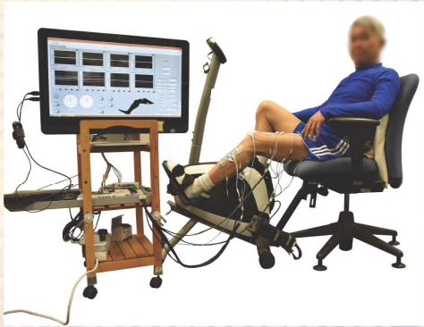
Structure of the interactive cycling system
