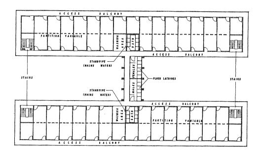
Floor Plan of Resettlement Building Mark II
