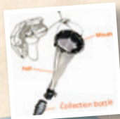
Fig.7 Structure of a plankton net
