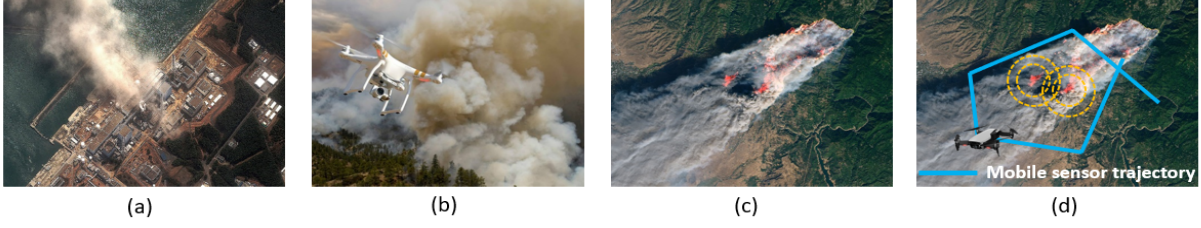
Fig. 1: Unmanned aerial vehicles can help determine radiation after incidents in nuclear facilities or during routine monitoring in (a), and localise wild fires in (b) and (c). The problem we consider in this paper is localising the diffusion sources and the trajectory of the mobile sensor from samples along unknown trajectories, as illustrated in (d).
