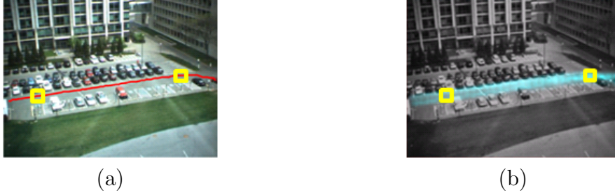
Figure 1-10: Learning motion patterns from identity co-occurrence. Identity co-occurrence means that two feature values are on the same trajectories and are related to the same object. (a) Two locations marked by yellow boxes are on the same trajectory. (b) Two locations marked by yellow boxes are in the same semantic region and thus they co-exist on many trajectories. Based on the identity co-occurrence information, a semantic region model with large distribution on both two locations can be learned.
