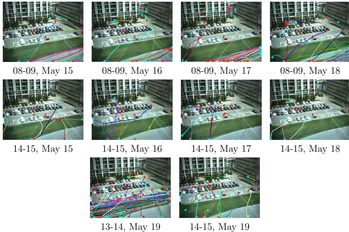
Figure 4-21: Abnormal trajectories in the parking lot scene detected at different time slices. The same threshold of data likelihood is used for all the slices. Between 7 o'clock and 8 o'clock in the morning everyday, many trajectories passing through the bottom right corner of the scene are detected as abnormal. There are not many trajectories of this activity happening in the morning. When they start to appear in a large number between 8 o'clock and 9 o'clock, they are detected as abnormal. Between 13 o'clock and 15 o'clock on May 16th, a worker was mowing the grass around this time. Many trajectories moving back and forth horizontally on the grass field are detected as an abnormality between 13 o'clock and 14 o'clock. However, after the model of this activity has been well learnt at this time slice, similar trajectories are not detected as abnormal in the next hour.
