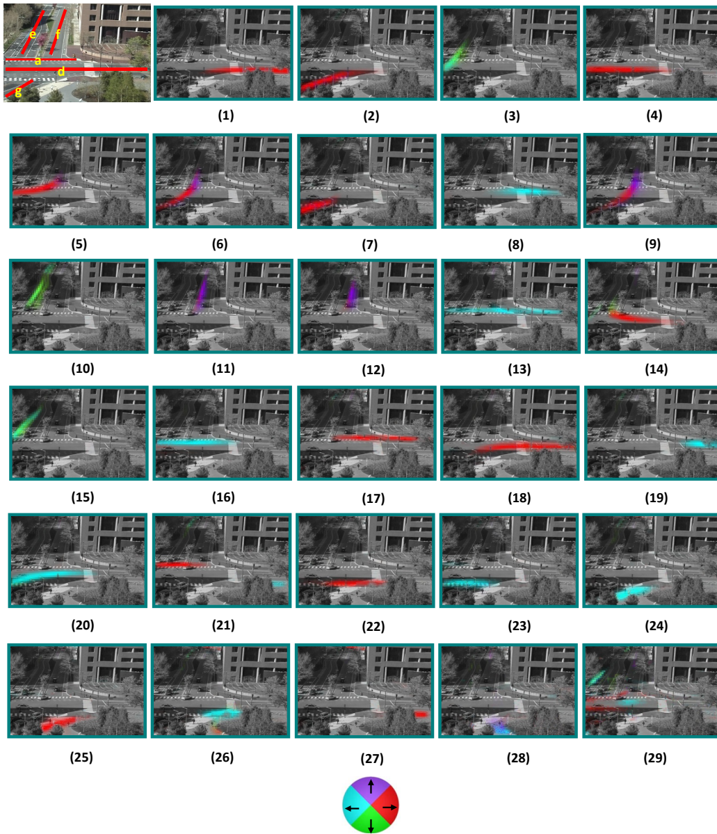
Figure 3-6: Distributions of 29 atomic activities (topics) discovered by our Dual-HDP models. Colors represent four quantized moving directions: red ( \rightarrow ), magenta ( \uparrow ), cyan ( \leftarrow ), and green ( \downarrow ). The intensity represents the density of distributions. The atomic activities are sorted according to how many moving pixels in the data set are assigned to them (from large to small). For convenience, we label roads and crosswalks as a, b, \dots in the first image. From these distributions, we can guess some activities happening in this scene, such as vehicles turning left (atomic activity 5 and 20), pedestrians crossing streets (atomic activity 13, 17, 21, 22 and 23), and vehicles crossing the intersection (atomic activity 6 and 9).
