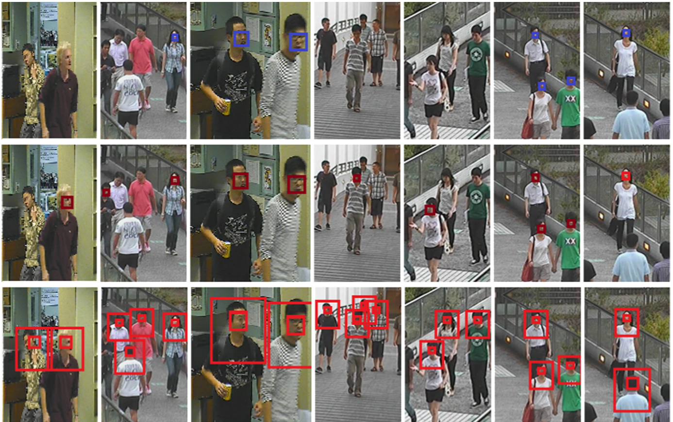
Fig. 16. Face detection results on surveillance frames. First row: Viola–Jones' results; second row: HeadHunter's results; last row: our results.
