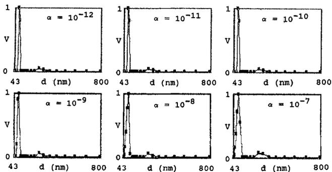
Fig. 3: Calculated volume distributions of a latex dispersion, which is a mixture of two narrowly distributed latexes ( $d_1 = 90$  nm and  $d_2 = 312$  nm with a volume ratio of  $V(d_1):V(d_2) = 95:5$ ) where 11 angles ( $40-90^\circ$ ) were used.
