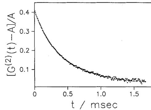
Fig. 1: Typical measured "normalized" intensity-intensity time correlation function  $C(n\Delta\tau, \theta)$  of a latex dispersion, which is a mixture of three narrowly distributed latexes ( $d_1 = 90$  nm,  $d_2 = 312$  nm,  $d_3 = 490$  nm with a volume ratio of  $V(d_1):V(d_2):V(d_3) = 7:2:1$ ).
