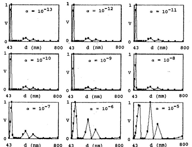
Fig. 5: Calculated volume distributions of a latex dispersion, which is a mixture of three narrowly distributed latexes ( $d_1 = 90$  nm,  $d_2 = 312$  nm and  $d_3 = 490$  nm with a volume ratio of  $V(d_1):V(d_2):V(d_3) = 7:2:1$ ), where six angles ( $40-90^\circ$ ) were used.
