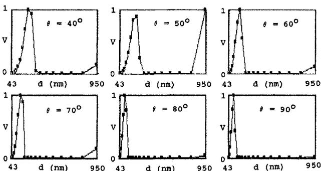
Fig. 4: Calculated volume distributions from the data in Figure 3, where only one scattering angle was used in each calculation.
