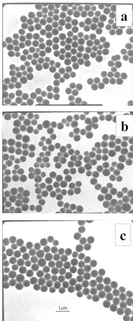
**Figure 1.** TEM images of S1 series nanoparticles prepared by the dispersion copolymerization of PNIPAAm macromonomer with St in mixed ethanol/water (7/3, v/v) solvents. (a) Sample S1-1; (b) S1-2; (c) S1-3 in Table II.
