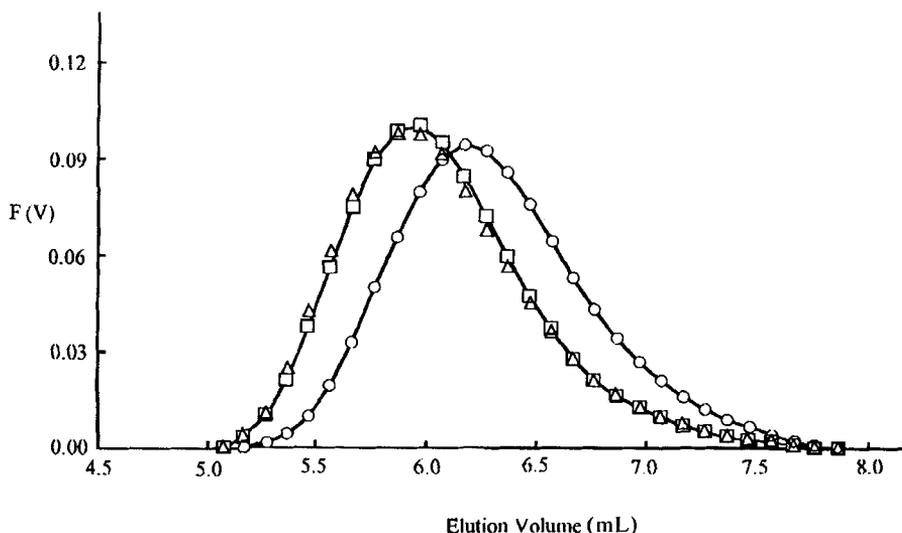
**FIG. 2.** SEC profiles of polystyrene in benzene:  $\square$ , original solution;  $\circ$ , after 200 times of freeze-thaw cycling;  $\triangle$ , after reheating the frozen solution.
