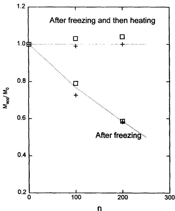
FIG. 3. Variation of apparent molar masses of polystyrene in solutions of different thermal history;  $n$  = number of freeze-thaw cycles. □, ratio of weight average molar masses; +, ratio of number-average molar masses.
