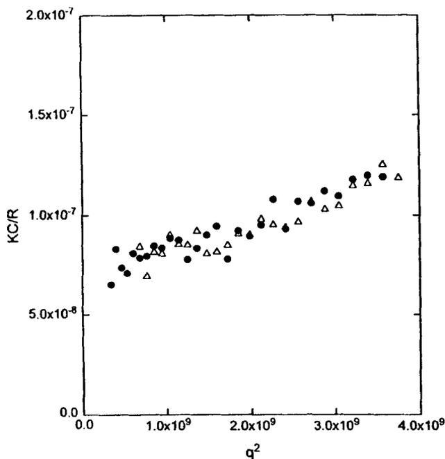
FIG. 5. SLS data of the solutions assuming different  $dn/dc$  values: ●, original solution,  $dn/dc = 0.114$ ; △, the solution after freeze-thaw cycling,  $dn/dc = 0.105$ .
