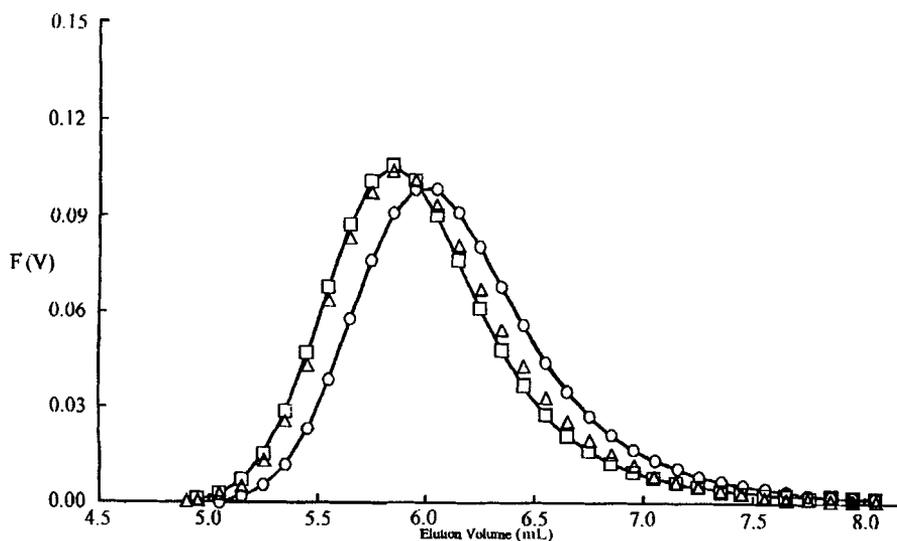
FIG. 1. SEC profiles of polystyrene in benzene:  $\square$ , original solution;  $\circ$ , after 100 times of freeze-thaw cycling;  $\triangle$ , after reheating the frozen solution.
