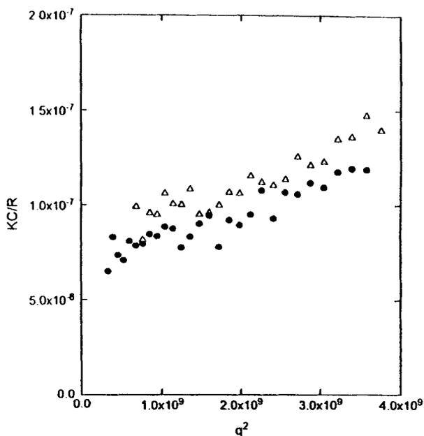
FIG. 4. SLS data for both original polystyrene-toluene solution (●) and after 61 freeze-thaw cycles (△) assuming the same  $dn/dC$  value (0.114) with the solution concentration of  $5.8 \cdot 10^{-3}$  g/mL.
