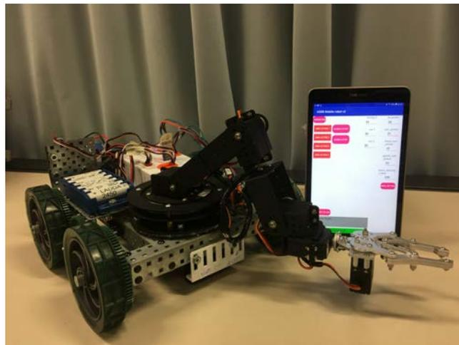
Figure 1: Developed robot and mobile application on tablet.
