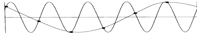
Figure 3.16 When a sine wave is sampled six times in five cycles, the observed sine wave has a much lower frequency than the original sine wave.
