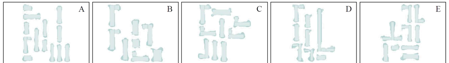
(b) Direct mask fracturing [20] results of Neural-ILT synthesized masks on benchmarks A-E.
