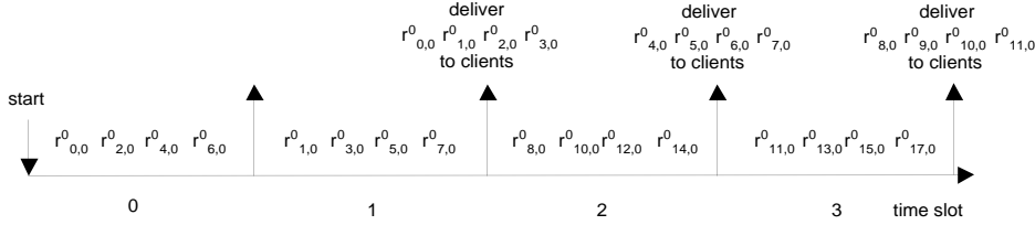
Fig. 5 Data retrieval and delivery process for VCR display at display resolution r' = 0
