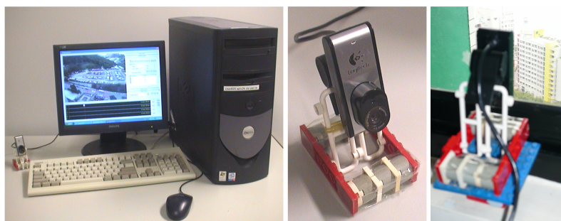
Fig. 7. The hardware setup: the whole setup (left) and the webcam (right).
