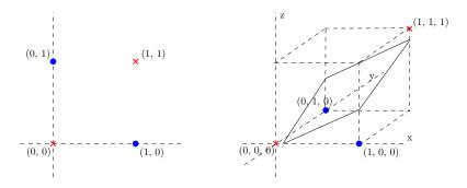
The right figure shows the 4 points after the transformation from a 2D point (x, y) to a 3D point (x, y, xy). The new dataset is linearly separable.
