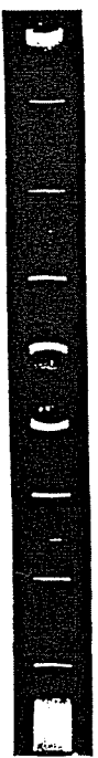
(a) Experimental geometry for a powder photograph. (b) A powder photograph of molybdenum taken with Co Kα radiation. The x-rays enter the camera through the hole in the center of the film and leave between the grids of the film. Note that the Kα-Kα₂ x-ray doublet (wavelengths 1.789 and 1.793 Å) is resolved in the back-scattered radiation near the entrance hole.
