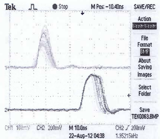
Fig. 2 Upper Trace: Ch 1, analog pulses going into the INPUT of the PCIT Lower Trace: Ch 2, standardized pulses coming from the MONITOR
