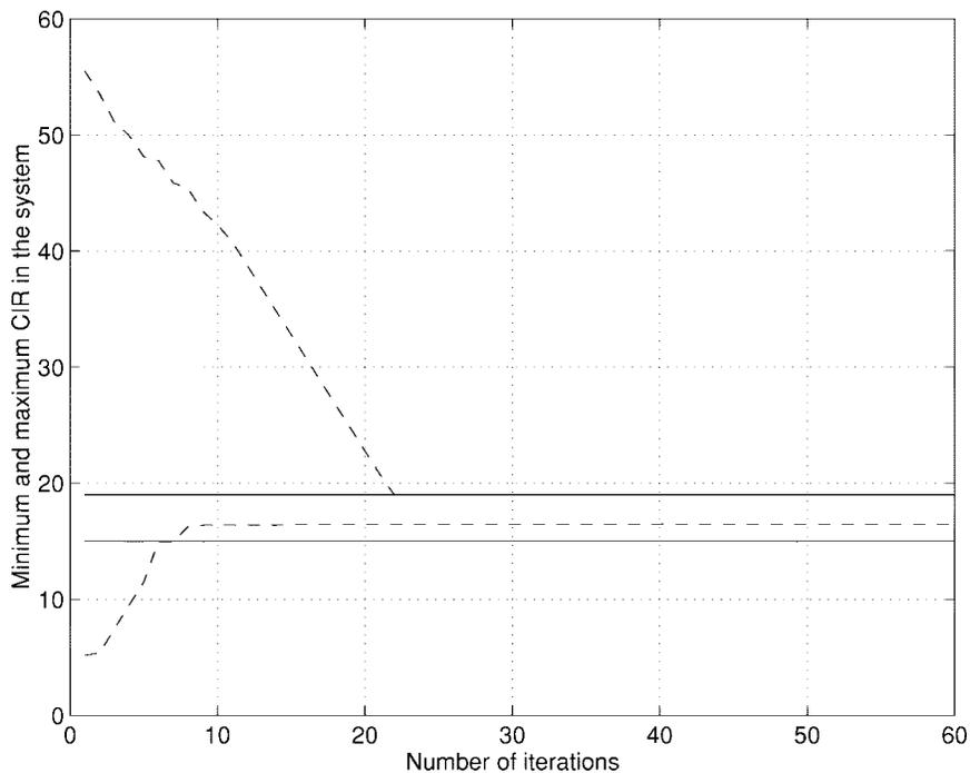
Fig. 3. Evolution of maximum and minimum CIR (decibels) with step size  $\delta = 2$  dB. The target window is also shown.
