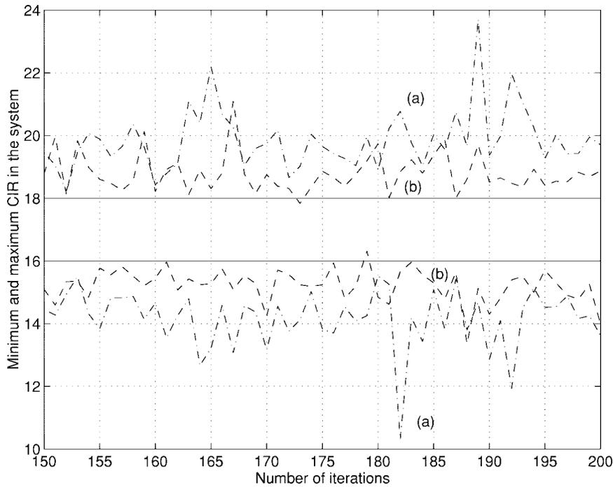
Fig. 5. Evolution of the maximum and minimum CIR (decibels) with CIR estimation error  $\sigma_w = 1$  dB. (a) Foschini's algorithm. (b) Fixed-step algorithm with step size  $\delta = 1$  dB. The target window of the fixed-step algorithm is also shown.
