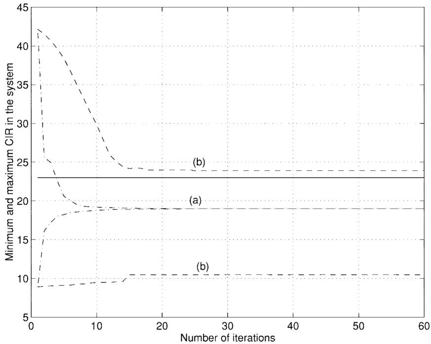
Fig. 4. Evolution of maximum and minimum CIR (decibels). (a) Foschini's algorithm. (b) Fixed-step algorithm with step size  $\delta = 1$  dB. The protection line is also shown.
