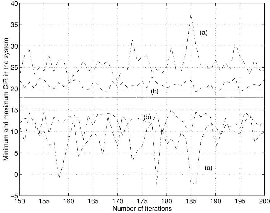
Fig. 6. Evolution of the maximum and minimum CIR (decibels) with CIR estimation error  $\sigma_w = 3$  dB. (a) Foschini's algorithm. (b) Fixed-step algorithm with step size  $\delta = 1$  dB. The target window of the fixed-step algorithm is also shown.
