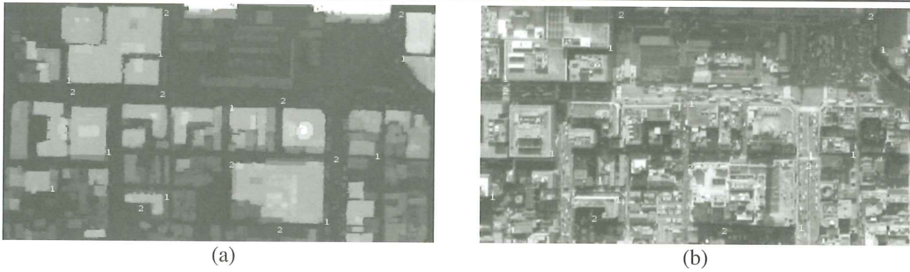
Figure 4. The study area (a part of Kyoto city), with no.1 for roof and no.2 for ground performing as control points. (a) Airborne laser data ; and (b) Aerial photograph
