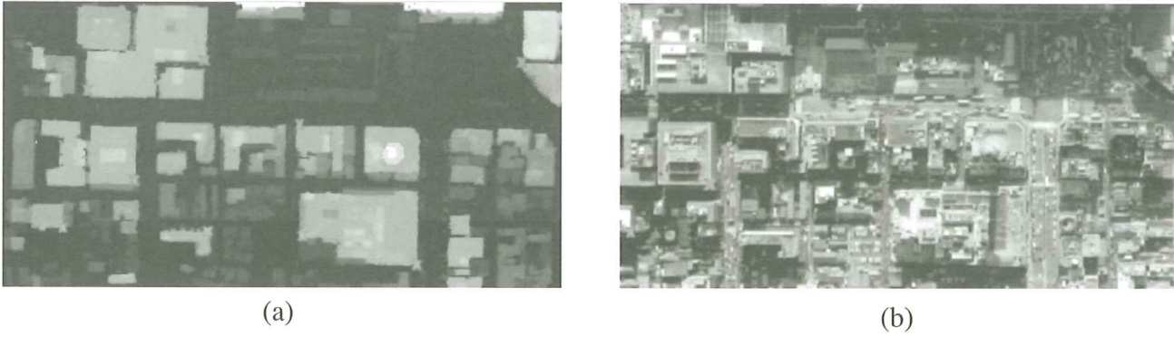
Figure 2. Control points allocation by X. (a) Control point on airborne laser data; and (b) Control point on aerial photograph
