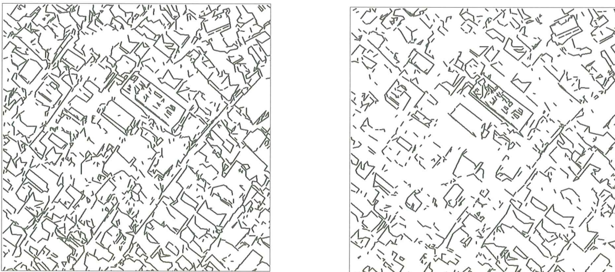
Figure 10. The result of line segmentation (SUSAN operator)
