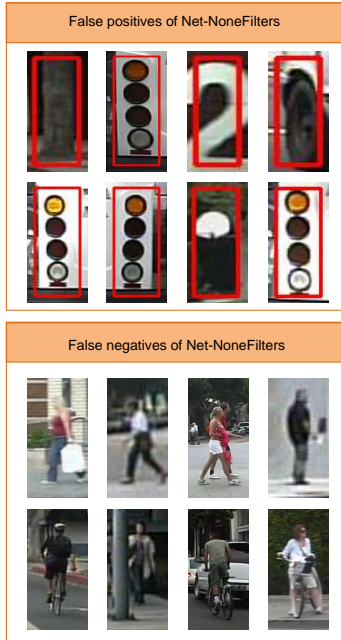
Figure 9. Detection results that are missclassified by DeepNet-NoFilter but correctly classified by ContDeepNet. Results are obtained from the 300 detection samples of the two approaches with the highest detection scores.
