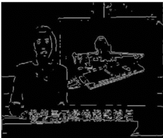
Figure 2: Frame edge filtered by Sobel filter
