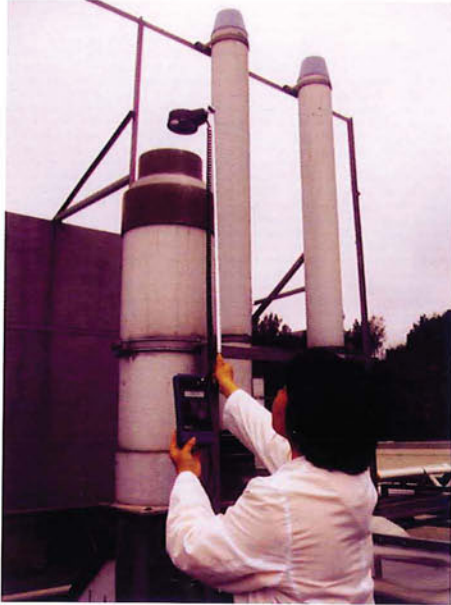
工作人員量度風櫃的排放風速 Measuring the discharge velocity of a fume cupboard exhaust stack
