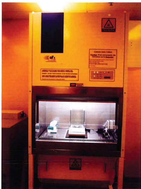
設於包玉剛爵士癌症中心的細胞毒性藥物量重櫃 A cytotoxic weighing cabinet at the Sir Yue Kong Pao Centre for Cancer
