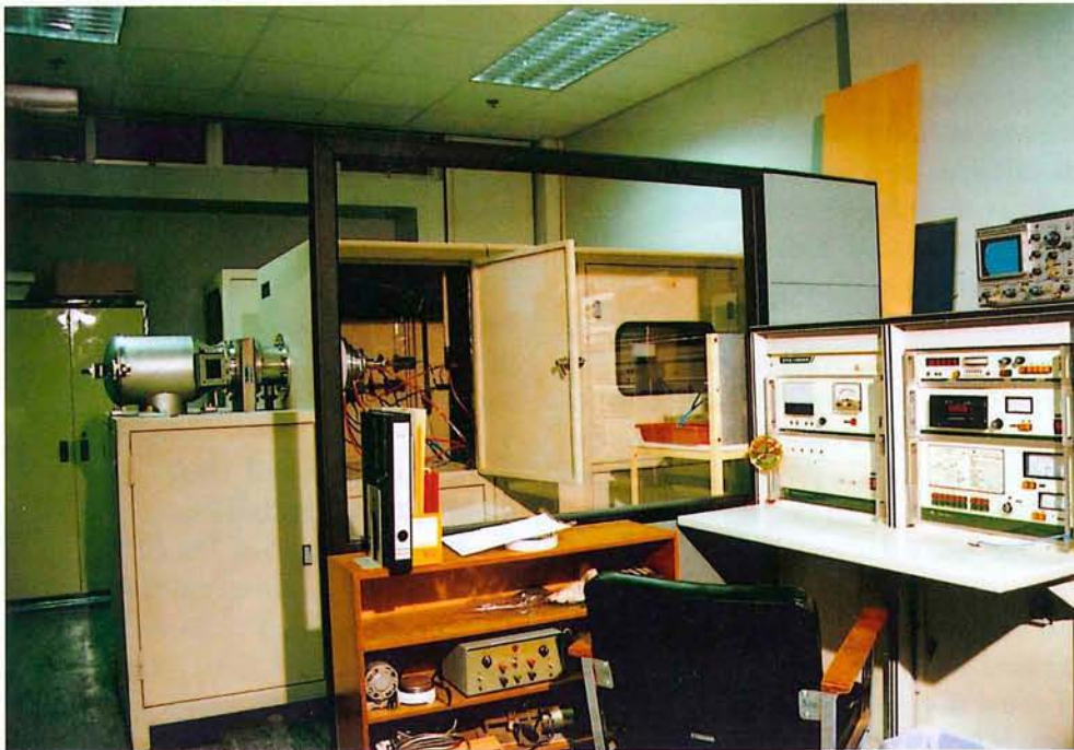
Fig. 1 The MEVVA implantation system in the Department of Electronic Engineering
