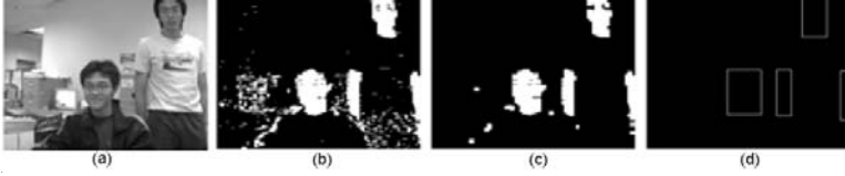
Fig. 2. The image for (a) original image, (b) binary skin mask, (c) binary skin mask after morphological operation and (d) face candidates are found
