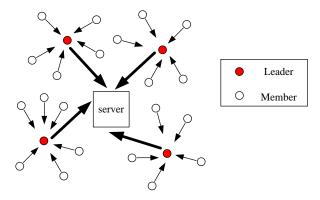
Figure 1: Reporting locations to cluster leaders using short-ranged communication has a much lower power consumption than making long-ranged communication with the server directly.
