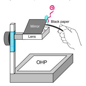
Figure 6: Smoking of a Black Paper Placed at the Image of the Filament
