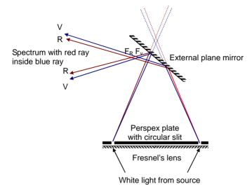
Figure 3b: Circular Spectrum Projected on a Screen With a Reversed Color Sequence
