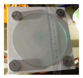
Note: Light comes from an OHP on the left with an incident angle about 85°. The central slotted weight is under the Perspex plate where Newton's rings are seen.
