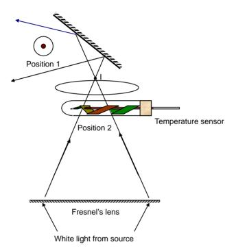
For safety, the level of projection lens should be adjusted before the experiment so that the image of the filament is formed just above the projection lens, and the boiling tube should be placed 10 to 15 cm either below the image (Position 1) or the same distance in front of the image (Position 2). In these positions, the light intensity will create a rise in temperature at a rate of 2-5 °C per minute, but not too strong to overheat the temperature sensor.
