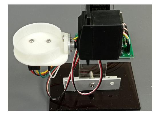
• The platform should be able to rotate 180 degree from left hand side to right hand side
