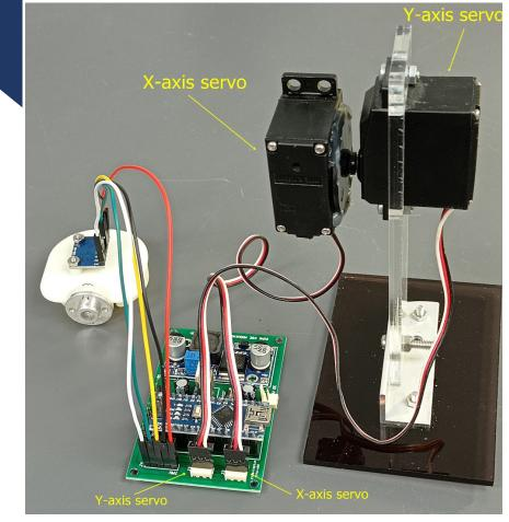
Connect 2 servo motors to the Arduino main board
