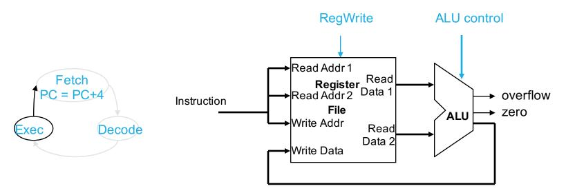
Note that Register File is not written every cycle (e.g. sw), so we need an explicit write control signal for the Register File
