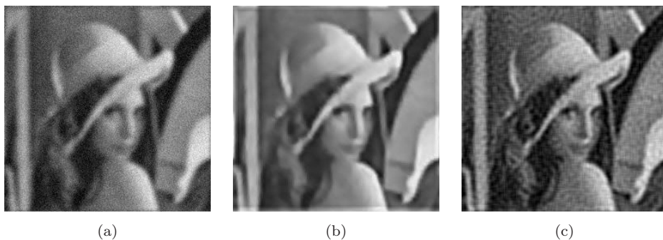
Fig. 4. Example of blind image restoration by WIPEM algorithm. (a) The blurred Lenna image, Gaussian type noise was added, (b) the restored image with WIPEM algorithm, and (c) the restored image using deconvblind function in Matlab image processing toolbox.
